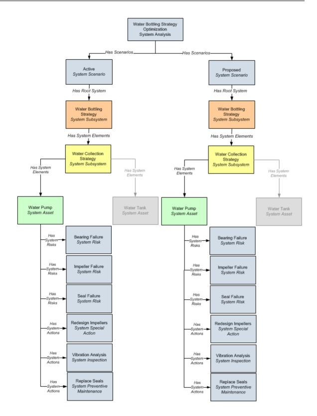
You can see that the *Water Pump* System Asset record is linked to three System Risk records. From the name of each System Risk record, you can infer the Risk record in ASM from which it was created. In addition, the *Water Pump* System
