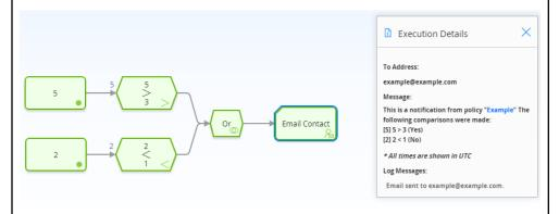
In this example, you can see that each node executed successfully. The logical result of the Or node is yes because the logical result of at least one incoming logic path results in a value of true passed to the Or node (that is, the result of the 5 > 3 Condition node is yes, which matches the logic path of the corresponding connection). Therefore, policy execution continues past the Or node.
