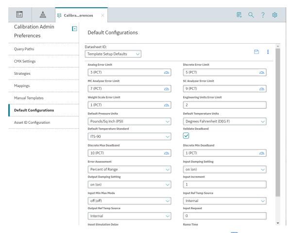
**Note:** As needed, you can modify the values in the required fields, and then select to save your changes. A value that has been modified in this section will be reflected in the respective Calibration Template datasheet.
