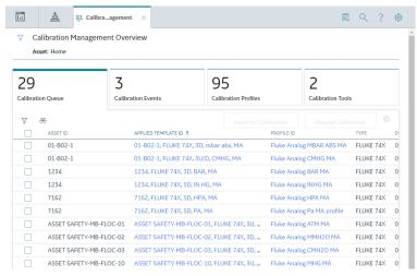
3. Select the check box that corresponds to the Calibration Task that you want to perform, and then, in the section, select **Manual Calibration**.
