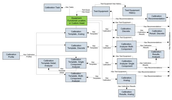
**Note:** In the diagram, boxes represent entity families and arrows represent relationship families that are configured in the baseline database. You can determine the direction of each relationship definition from the direction of the arrow head: the box from which the arrow originates is the predecessor, and the box to which the arrow head points is the successor.
