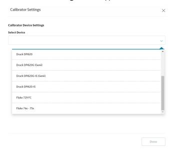
4. In the **Select Device** box, select Fluke 74X - 75X or Fluke 729 FC.
