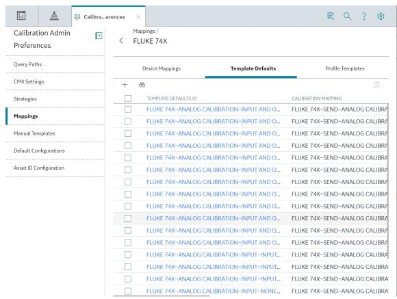
5. In the **Template Defaults ID** column, select the link for the Template Default that you want to access. The datasheet for the selected Template Default appears.
