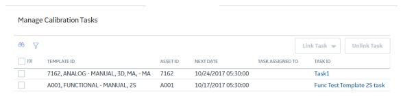
**Note:** You can also access the **Manage Calibration Tasks** page from the Calibration Profile datasheet. In the **Calibration Profiles** section, select a link in the **PROFILE ID** column to access the Calibration Profile datasheet, and then select **Manage Tasks**.
