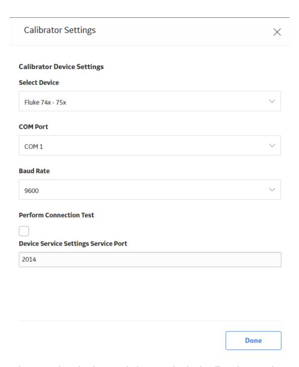
5. In the **COM Port** box, select the communication port number that the calibrator is connected to.
