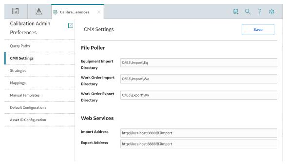
3. In the **File Poller** section, set the following folder paths that are used to perform calibration using CMX software:
