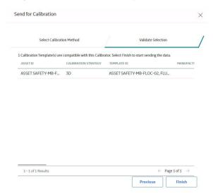
**Note:** If the selected calibration queue records have not been mapped to the correct device, when you select **Next**, the Calibration Templates will not be loaded and the **Finish** button will be disabled.
