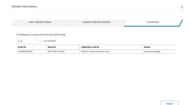
After receiving the calibration data, GE Digital APM creates a Calibration record for each calibration that you have selected. If you have used a documenting process calibrator for calibration, then the fields in the **Test Equipment** section of each Calibration record created are populated with the details of the calibrator.
