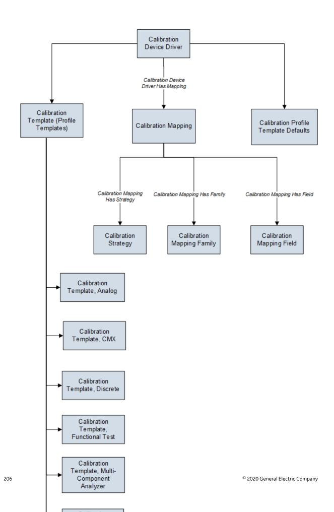
**Note:** In the diagram, boxes represent entity families and arrows represent relationship families that are configured in the baseline database. You can determine the direction of the each relationship definition from the direction of the arrow head: the box from which the arrow originates is the predecessor, and the box to which the arrow head points is the successor.
