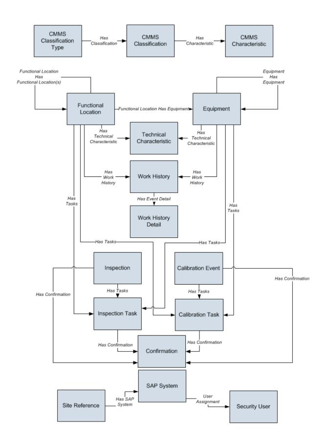
Note: In the diagram, boxes represent entity families and arrows represent relationship families that are configured in the baseline database. You can determine the direction of the each relationship definition from the direction of the arrowhead: the box from which the arrow originates is the predecessor, and the box to which the arrow head points is the successor.
