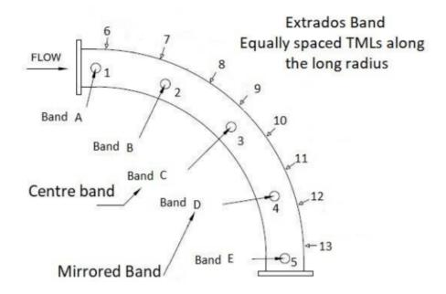
The following diagram illustrates the bands that can exist on a mitered elbow.
