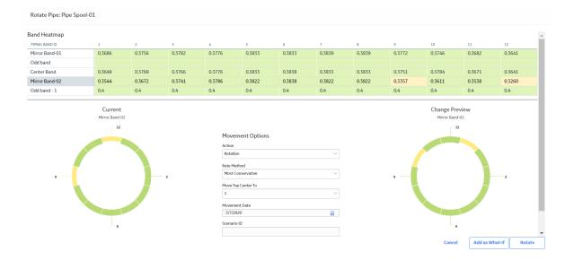
The **Band Heatmap** section contains the heat maps for each band on the Pipe Spool-01 component. Since the Mirror Band-02 band is selected, the heat map for that band appears in the widgets that display the positions of each TML before and after the rotation or flip.
