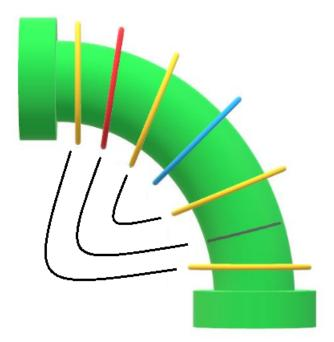
The bands colored yellow are mirrored bands, and the band colored blue is the center band. The band colored red is an odd band. When the elbow is flipped, the TMLs on the odd band move to a different location on the elbow, where a band did not previously exist.
