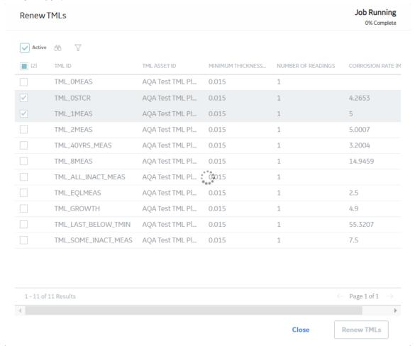
**Tip:** The renewal process continues even if you close the **Renew TMLs** window. You can view the progress of the job from the Schedule Logs. In case any TML fails to renew, the job is placed in the **Failed** section of the **Schedule Logs** page.
