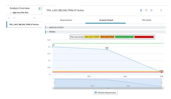
**Note:** By default, the Trends graph displays data based on the thickness measurements and Controlling Corrosion Rate for the TML.
