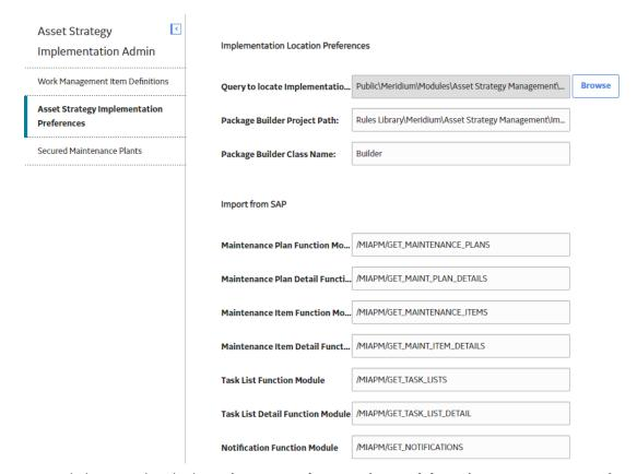
3. As needed, enter values in the Maintenance Plan Function Module, Maintenance Item Function Module, Task List Function Module, and Notification Function Module boxes.
