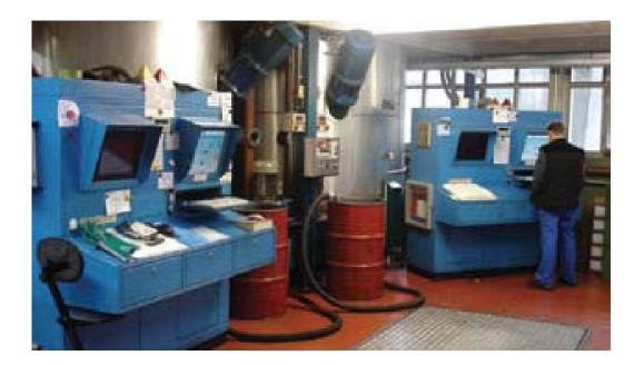
Using CIMPLICITY, the production staff member logs his system along with the starting time and temperature onto the energy management system of the power station. After the last heating cycle of a batch, the system automatically logs off again.
