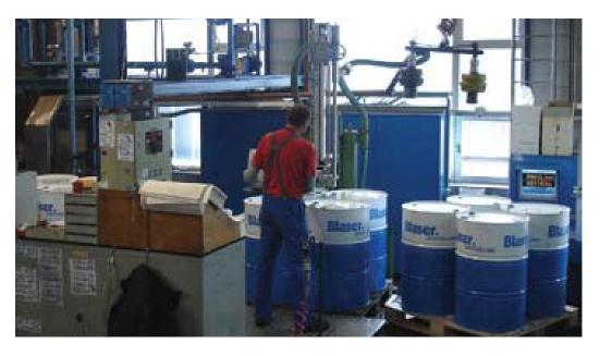
Thanks to the visualization, for example, in the filling station, the majority of the system faults can be remedied without interrupting the filling process.
