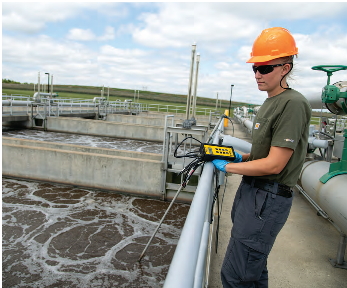
Caitlin Raasch uses a solids meter (YSI, a Xylem brand) to measure mixed liquor suspended solids levels in an aeration basin.
