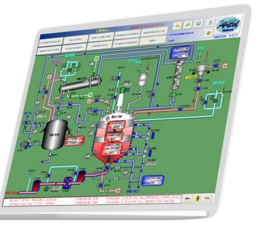
The material stocked in silos is conveyed by means of a compressed air tube system to the hoppers, and from there to gravimetric dispensers, which in turn feed the right amount of material into the reactor. The molten product from the reactor is extruded, cut into granules, and finally carried by another conveyor system to the packaging line, where it is put into bags or boxes.
