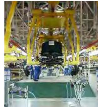
stations permitting line-side direct delivery of parts; a centralized nerve center; and options for future expansion without interrupting production. Three automated conveyor systems complete the efficient assembly process.
