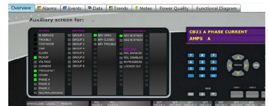
*Equipment controls in iPower are provided via universal control and information containers for each device called Tab Displays. These provide convenient access to all data, controls, and user material for each device.*
