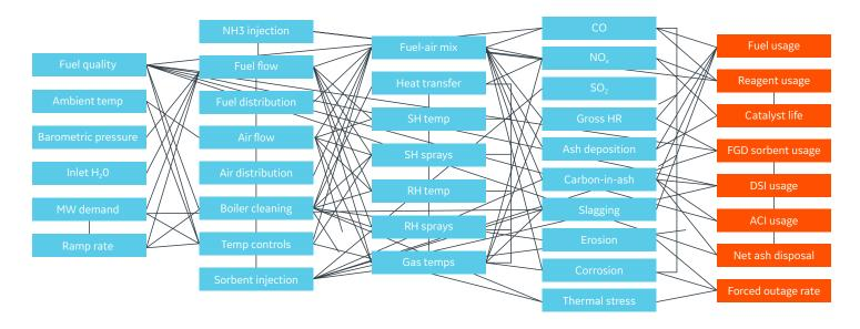
By making improvements from the fuel supply, within the boiler, and across the balance of plant, there is potential to incrementally impact efficiency, flexibility, availability, and emissions.
