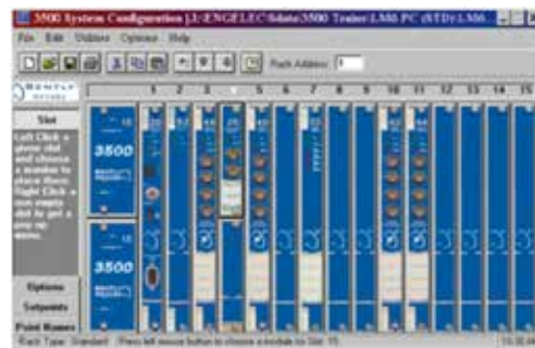
Bently Nevada Vibration System Display
