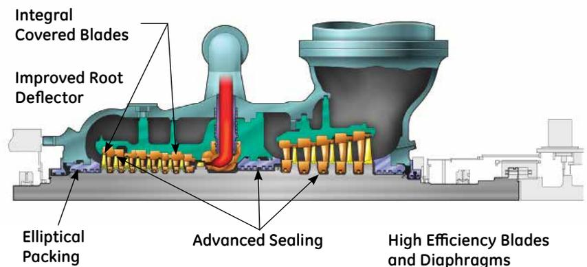
Cross section of typical Dense Pack Technology for combined HP/IP Section
