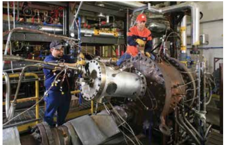
Figure 8 – Full combustion chamber test stand at GE's Global Research facility
