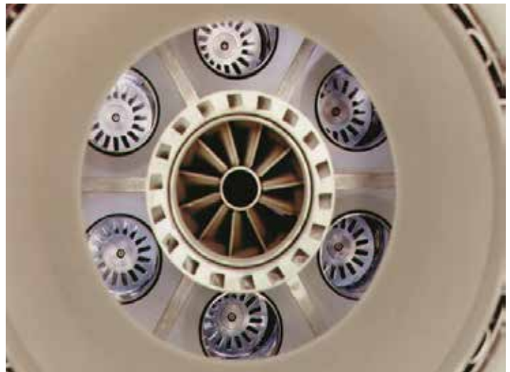
Figure 11 – DLN1 combustion system
