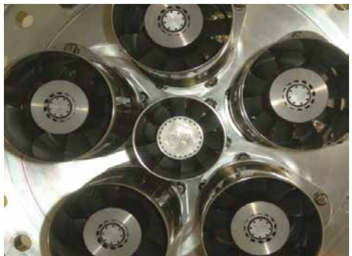
Figure 12 – DLN2.6+ combustion system
