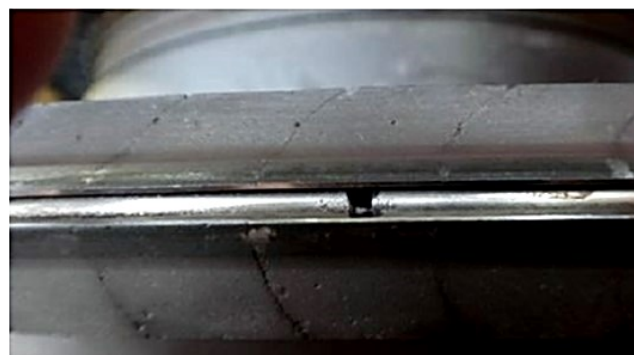
Fig. 5: Repair process: rolling-in the wire; quality check
