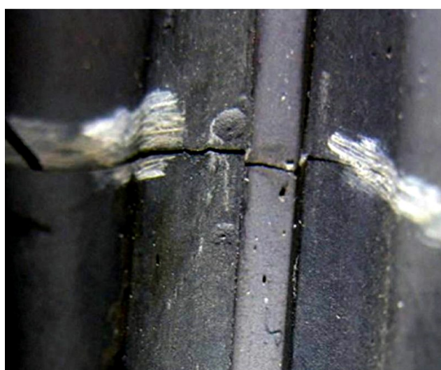
Fig. 1: AEG Kanis G25 turbine control stage, damaged damping wire.
