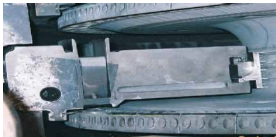
Fig. 1. Dished diaphragm before refurbishment
