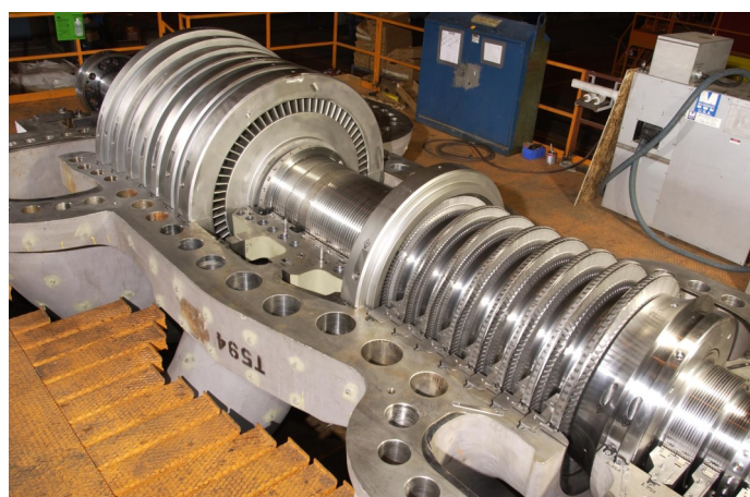
Fig. 2. D11 steam turbine HP/IP rotor after diaphragm refurbishment and reassembly
