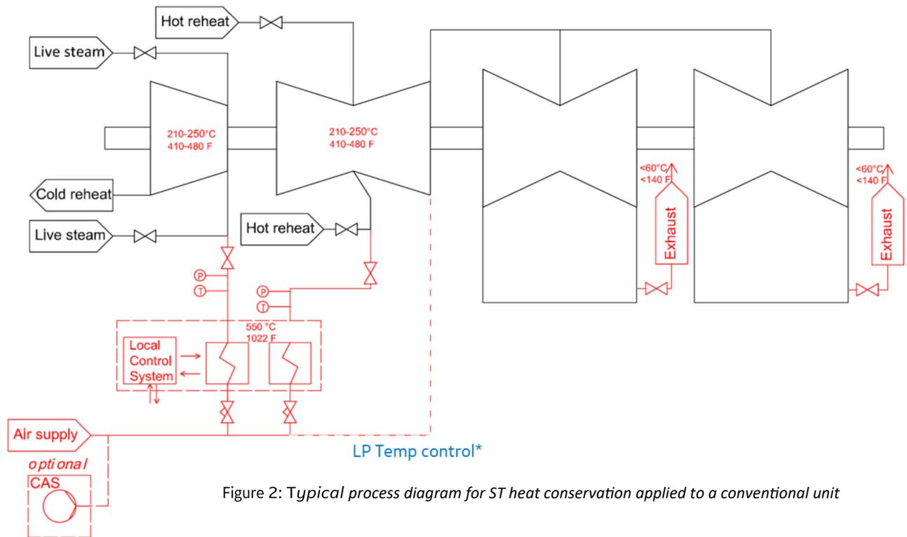
Figure 2: Typical process diagram for ST heat conservation applied to a conventional unit
