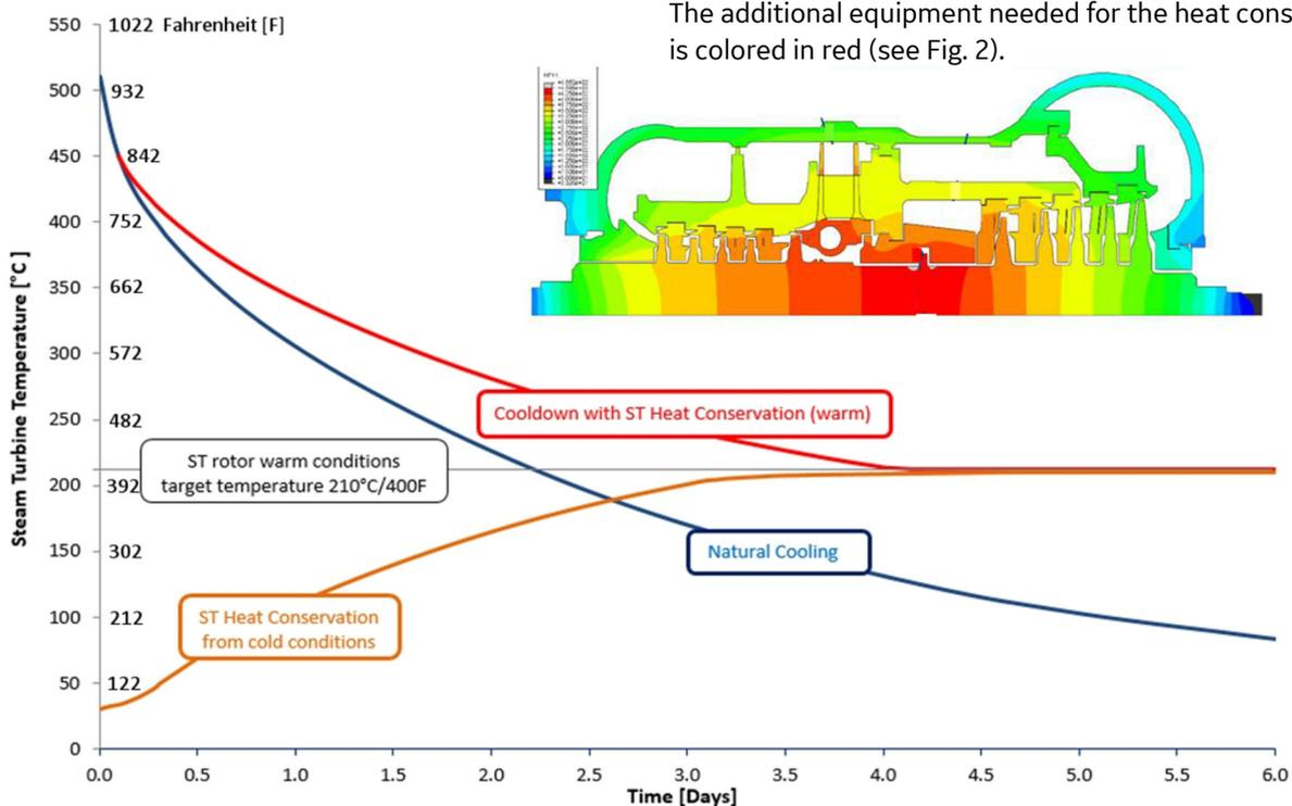
Figure 1: Typical ST metal temperature profiles after shut-down with and without HCS and applying HCS from a cold start condition.
