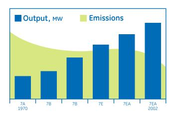
Improvements in design, materials, cooling, coatings and sealing have yielded a significant increase in output while reducing emissions.
