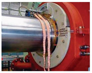
Installed shaft grounding strips on DE bearing pedestal
