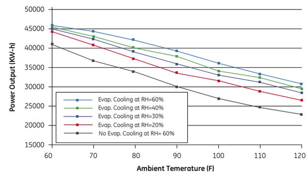
Increased Power Output of LM6000 Engine at Various Humidities.
