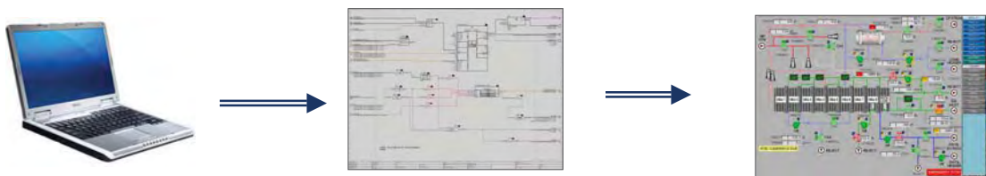
Figure #4 PC based controller emulation allows development of logic and screens
