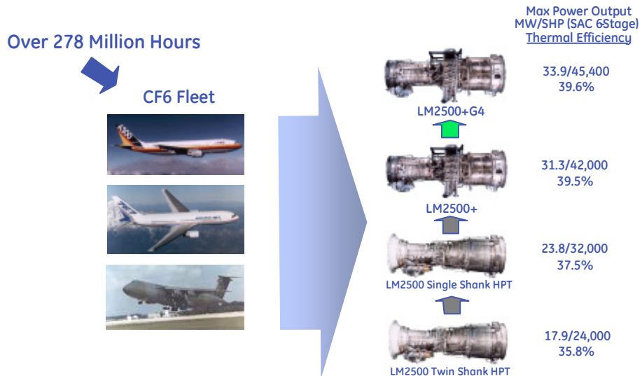
Figure 3. LM2500+G4 Gas Turbine Heritage
