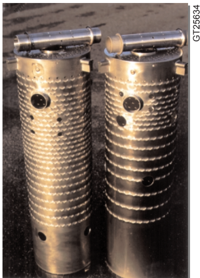
Figure 22. Louvered low NO x lean head end combustion liners
