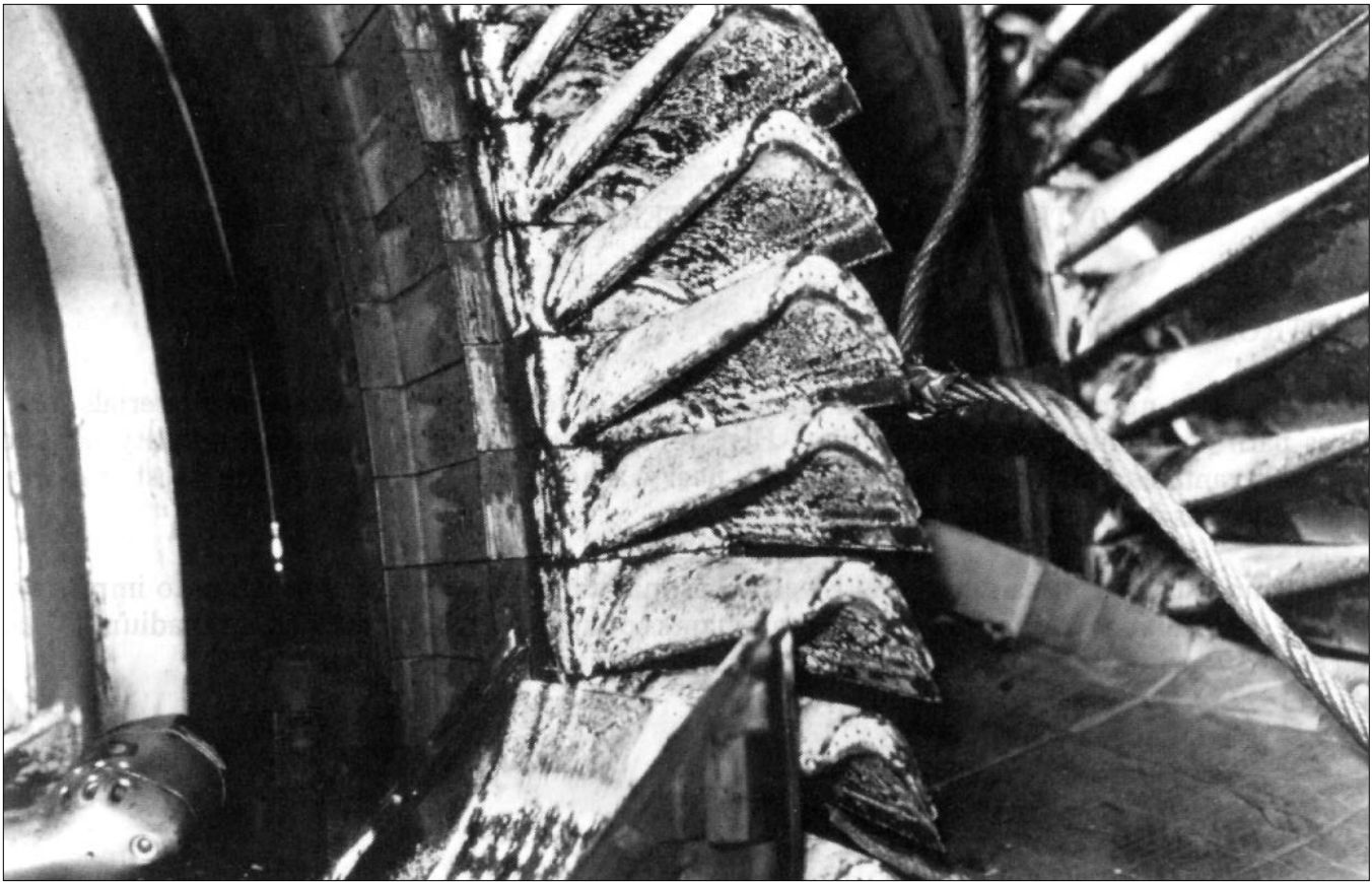
Figure 10. Deposits of sea salt on MS7001 first-stage nozzle partitions and buckets. Note condensates in locally cooled surfaces
