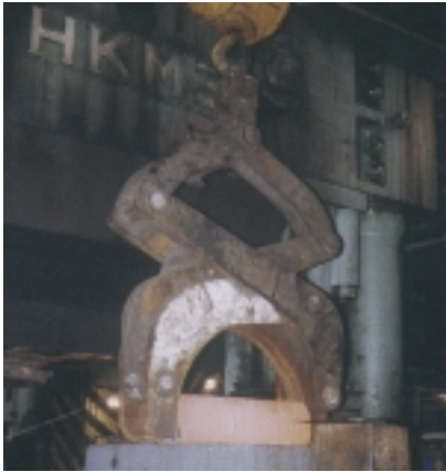
Figure 27. 7FA IN-706 turbine forging
