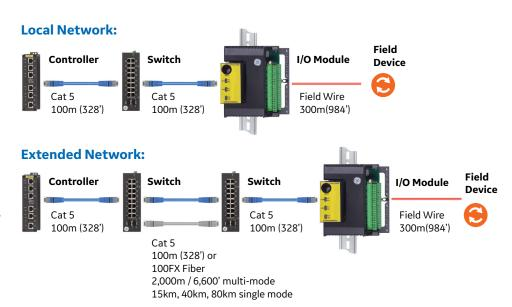
The distributed Ethernet architecture allows for enhanced connectivity and flexibility. Ethernet improves lifecycle management by enabling replacement or upgrade of individual components. The "future-proof" architecture of the Mark VIe platform enables a control system lifetime engineered to exceed expectations.
