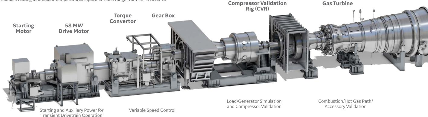
GE's 7HA.03 Gas Turbine has unmatched efficiency available at >64% net combined-cycle efficiency; higher than any other competing 60 Hz technology today.
