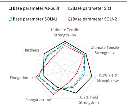
Spider Plot is generated by normalizing typical material data (containing both horizontal and vertical data) against a range defined for each material family. For **Stainless Steels**, the ranges are as follows: UTS: 0-750 MPa, 0.2%YS: 0-650 MPa, Elongation: 0-70 %, Hardness: 0-250 HV10
