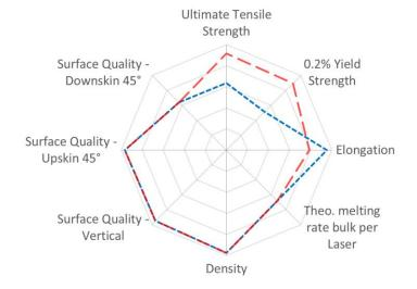
Spider Plot is generated by normalizing typical material data (containing both horizontal and vertical data) against a range defined for each material family. For nickel-based superalloys, the ranges are as follows: UTS: 0-1600 MPa, 0.2%YS: 0-1400 MPa, Elongation: 0-40 %, Density: 0-100 %, Productivity: 5-30 cm $^3$ /h, Surface Quality (all): 70-5  $\mu$ m
