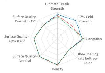
Spider Plot is generated by normalizing typical material data (containing both horizontal and vertical data) against a range defined for each material family. For **Stainless Steels**, the ranges are as follows: UTS: 0-750 MPa, 0.2%YS: 0-600 MPa, Elongation: 0-60 %, Density: 99-100 %, Theo. melting rate bulk per Laser: 5-30 cm $^3$ /h, Surface Quality (all): 50-5  $\mu$ m
