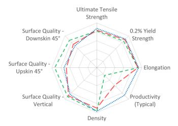
Spider Plot is generated by normalizing typical material data (containing both horizontal and vertical data) against a range defined for each material family. For **Ti-64**, the ranges are as follows: UTS: 600-1100 MPa, 0.2%YS: 500-1000 MPa, Elongation: 0-20 %, Density: 99-100 %, Productivity: 0-70 cm³/h, Surface Quality (all): 50-5 μm
