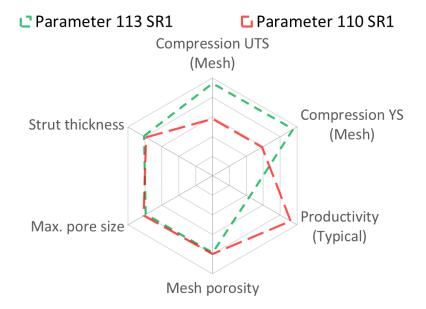
Spider Plot is generated by normalizing typical material data (containing both horizontal and vertical data) against a range defined for each material family. For **Ti-64 (mesh parameter)**, the ranges are as follows: Compression UTS (Mesh): 0-110 MPa, Compression YS (Mesh): 0-85 MPa, Density: 0-80%, Productivity: 5-40 cm³/h, Max. Pore Size: 0-600 µm, Strut Thickness: 0-300 µm
