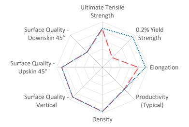
Spider Plot is generated by normalizing typical material data (containing both horizontal and vertical data) against a range defined for each material family. For **Tool Steel** alloys, the ranges are as follows: UTS: 900-2000 MPa, 0.2%YS: 600-1600 MPa, Elongation: 0-10 %, Density: 99-100 %, Productivity: 5-30 cm³/h, Surface Quality (all): 40-5 μm
