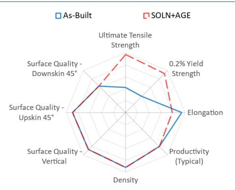
Spider Plot is generated by normalizing typical material data (containing both horizontal and vertical data) against a range defined for each material family. For copper alloys, the ranges are as follows: UTS: 0-600 MPa, 0.2%YS: 0-500 MPa, Elongation: 0-50%, Density: 0-100%, Productivity: 5-30 cm<sup>3</sup>/hr, Surface Quality (all): 40-5 μm
