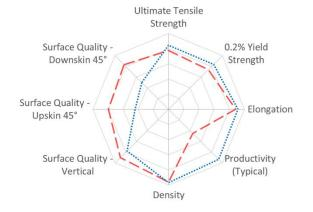
Spider Plot is generated by normalizing typical material data (containing both horizontal and vertical data) against a range defined for each material family. For **Ti-64**, the ranges are as follows: UTS: 600-1100 MPa, 0.2%YS: 500-1000 MPa, Elongation: 0-20 %, Density: 99-100 %, Productivity: 0-100 cm<sup>3</sup>/h, Surface Quality (all): 50-5 μm
