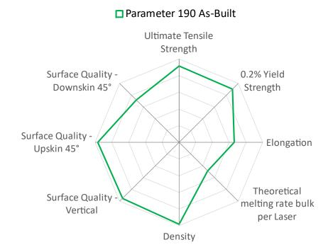
Spider Plot is generated by normalizing typical material data (containing both horizontal and vertical data) against a range defined for each material family. For **Cobalt Alloys**, the ranges are as follows: UTS: 0-1400 MPa, 0.2%YS: 0-900 MPa, Elongation: 0-60 %, Density: 99-100 % and Surface Quality (all): 40-5 µm.
