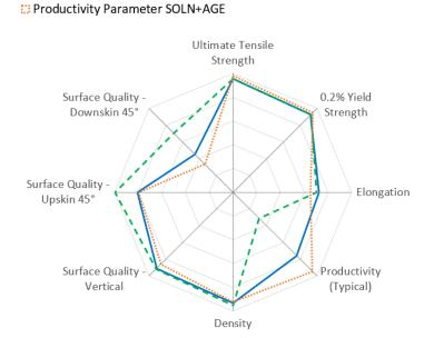
Spider Plot is generated by normalizing typical material data (containing both horizontal and vertical data) against a range defined for each material family. For **Precipitation Hardening Steels**, the ranges are as follows: UTS: 0-1500 MPa, 0.2%YS: 0-1400 MPa, Elongation: 0-30 %, Density: 99-100 %, Productivity: 5-30 cm<sup>3</sup>/h, Surface Quality (all): 40-5 μm
