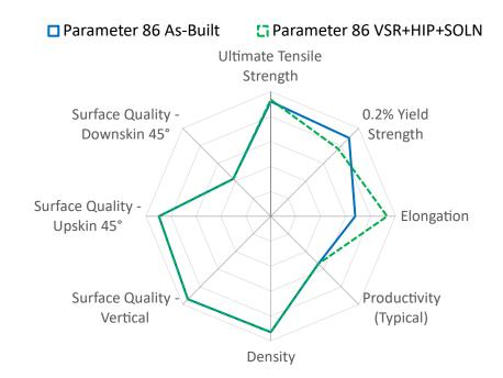
Spider Plot is generated by normalizing typical material data (containing both horizontal and vertical data) against a range defined for each material family. For **Cobalt Alloys,** the ranges are as follows: UTS: 0-1400 MPa, 0.2%YS: 0-900 MPa, Elongation: 0-60 %, Density: 99-100 %, Productivity: 5-30 cm<sup>3</sup>/h, and Surface Quality (all): 40-5 µm.
