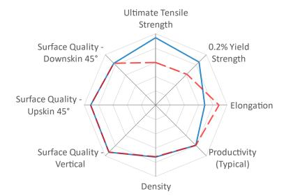
Spider Plot is generated by normalizing typical material data (containing both horizontal and vertical data) against a range defined for each material family. For **Aluminum Alloys**, the ranges are as follows: UTS: 0-500 MPa, 0.2%YS: 0-300 MPa, Elongation: 0-20 %, Density: 99-100 %, Productivity: 5-30 cm³/h, Surface Quality (all): 40-5 μm
