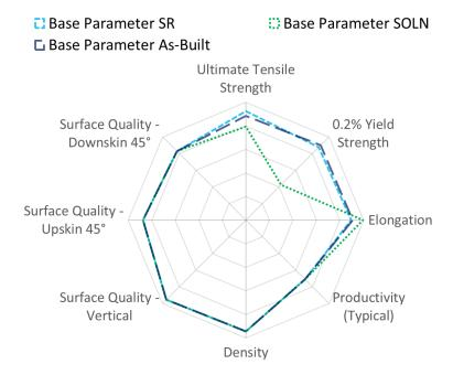
Spider Plot is generated by normalizing typical material data (containing both horizontal and vertical data) against a range defined for each material family. For **Stainless Steels**, the ranges are as follows: UTS: 0-750 MPa, 0.2%YS: 0-600 MPa, Elongation: 0-60 %, Density: 99-100 %, Productivity: 5-30 cm³/h, Surface Quality (all): 50-5 µm
