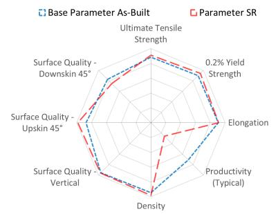
Spider Plot is generated by normalizing typical material data (containing both horizontal and vertical data) against a range defined for each material family. For **Stainless Steels**, the ranges are as follows: UTS: 0-750 MPa, 0.2%YS: 0-600 MPa, Elongation: 0-60 %, Density: 99-100 %, Productivity: 5-30 cm<sup>3</sup>/h, Surface Quality (all): 50-5 µm
