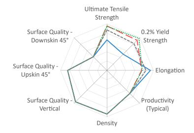
Spider Plot is generated by normalizing typical material data (containing both horizontal and vertical data) against a range defined for each material family. For nickel-based superalloys, the ranges are as follows: UTS: 0-1600 MPa, 0.2%YS: 0-1400 MPa, Elongation: 0-40 %, Density: 0-100 %, Productivity: 5-30 cm³/h, Surface Quality (all): 70-5 µm
