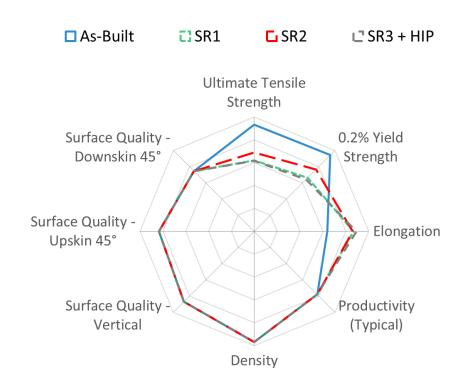
Spider Plot is generated by normalizing typical material data (containing both horizontal and vertical data) against a range defined for each material family. For **Ti-64**, the ranges are as follows: UTS: 600-1250 MPa, 0.2%YS: 500-1100 MPa, Elongation: 0-20 %, Density: 99-100 %, Productivity: 5-30 cm<sup>3</sup>/h, Surface Quality (all): 50-5 µm
