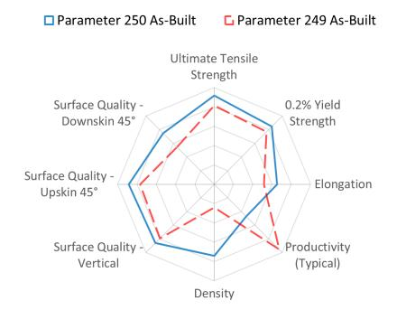
Spider Plot is generated by normalizing typical material data (containing both horizontal and vertical data) against a range defined for each material family. For **Aluminum Alloys**, the ranges are as follows: UTS: 0-500 MPa, 0.2%YS: 0-300 MPa, Elongation: 0-20 %, Density: 99-100 %, Productivity: 5-60 cm<sup>3</sup>/h, Surface Quality (all): 40-5 μm
