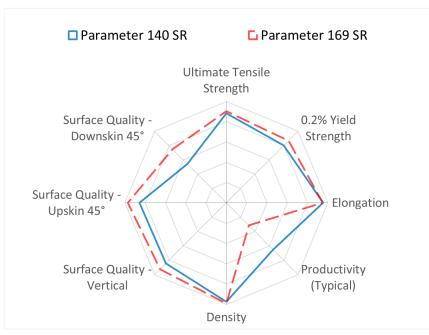
Spider Plot is generated by normalizing typical material data (containing both horizontal and vertical data) against a range defined for each material family. For nickel-based superalloy **Nickel 625**, the ranges are as follows: UTS: 0-1050 MPa, 0.2%YS: 0-750 MPa, Elongation: 0-50 %, Density: 99-100 %, Productivity: 5-30 cm<sup>3</sup>/h, Surface Quality (all): 40-5 µm
