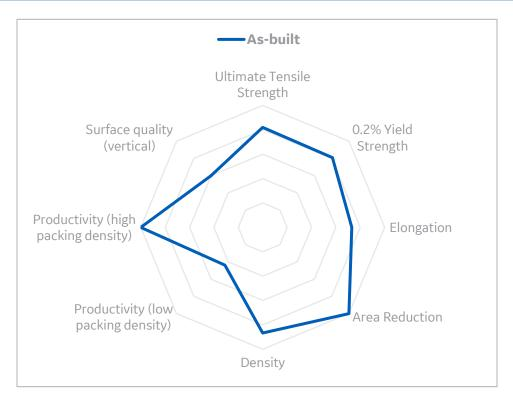
Spider Plot is generated by normalizing typical material data (containing both horizontal and vertical data) against a range defined for each material family. For Titanium Alloys, the ranges are as follows: UTS: 0-1200 MPa, 0.2%YS: 0-1100 MPa, Elongation: 0-20 %, Density: 99-100 %, Productivity: 5-30 cm<sup>3</sup>/hr, Surface Quality (all): 50-4 µm
