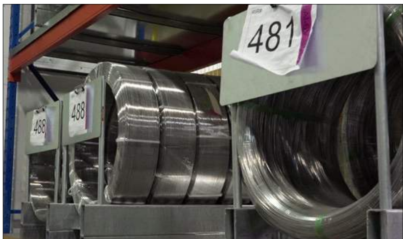
Fig. 4 Titanium wire feedstock used in the plasma atomisation process
