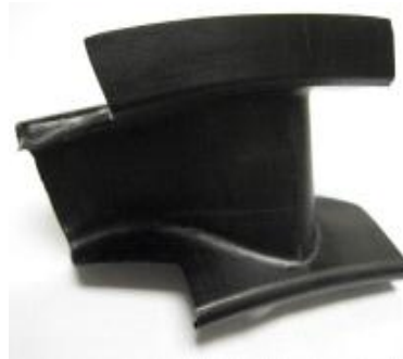
Ceramic Matrix Composites +300°F temperature capability vs. superalloys
