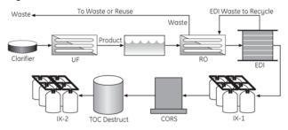
Figure 4: Power Plant 2: Train of Unit Operations
