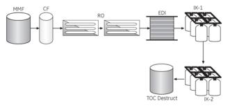
Figure 5: Microchip Plant Water Treatment System
