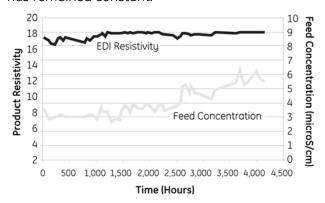
Figure 10: Microelectronics Plant Unit A Product Resistivity vs. Time
