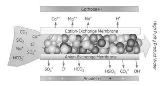
Figure 1: EDI Flow Schematic
